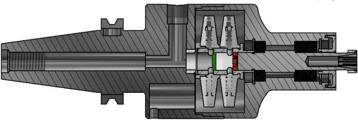
Green Position - Single Turbine Mode. Red Position - Double Turbine Mode.
