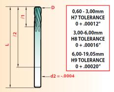
All reamers have a 45° chamfer lead Ø.0236" to .0929 = 4 flutes, Ø.0933" to .5138= 6 flutes, 10 degree left spiral/right hand cut for through holes.
