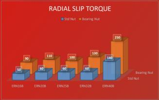
ER32 standard nut locked at 100 ft/lbs using a 1/2" carbide test arbor, the arbor slips at 60 ft/lbs of radial torque, using a Pioneer Bearing Nut the arbor slipped at 130 ft/lbs of radial toque.
